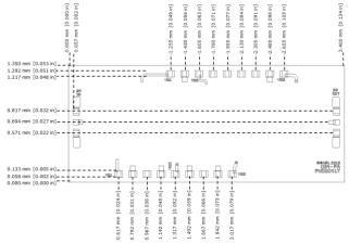
DC Bond Pads are 0.1mm<sup>2</sup>; Bond pad locations shown from die etch to pad center.
